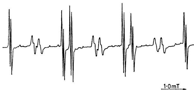
FIGURE 2 E.s.r. spectrum of the radical anion -\text{O}_2\text{C}\cdot\text{CH}_2\cdot\text{CH}(\text{CO}_2^-)\cdot\text{CH}_2\cdot\text{NO}_2^- at 20^\circ
